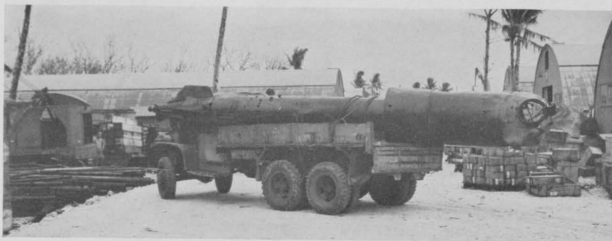
Human Torpedo, ULITHI Type—November 1944, showing access hatch.
