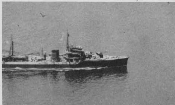
MIKURA Class, Rabaul—November 2, 1943. Note twin shield mount forward, open twin mount aft.
