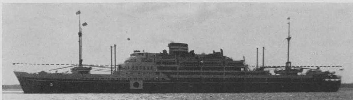
ARGENTINA MARU before conversion to CVE KAIYO. Dotted line represents probable location of flight deck.
