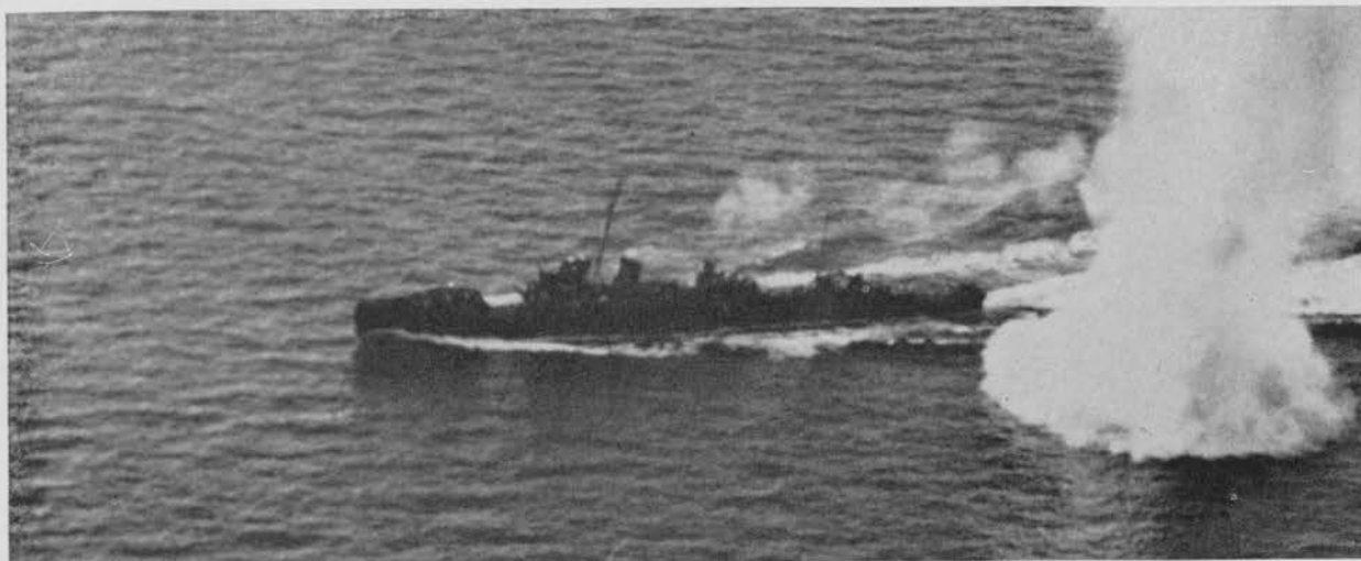
KURI—WAKATAKE Class—March 30, 1944. Note forward torpedo tubes removed.
